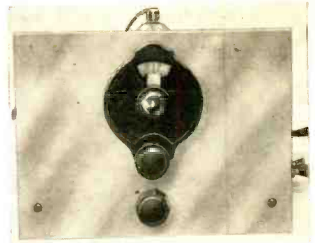
The 1-tube R.F. booster viewed from the front.
