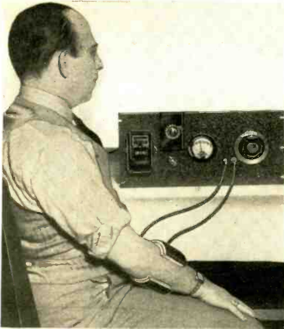
The short-wave diathermy oscillator in operation, showing how electrodes are placed for treating an ailment of the arm.
