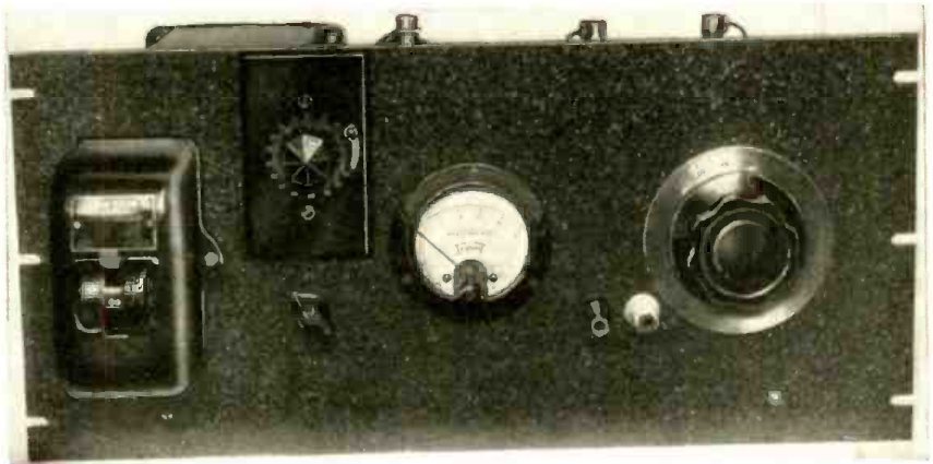
Front view of the S-W Diathermy apparatus, showing the "dosage meter," adjustable time switch and the circuit-breaker at the extreme left. The control for the tuning condenser in the patient's circuit is shown at the right.
